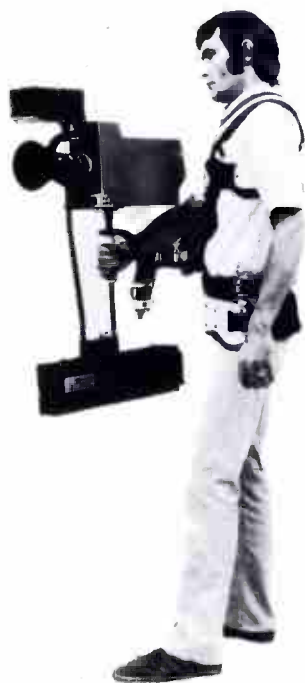
The CP/TK-76 Stabilized Video Camera System produces jitter free pictures.
